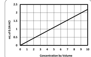
Concentration = Refractive Index X Refractometer Multiplier
